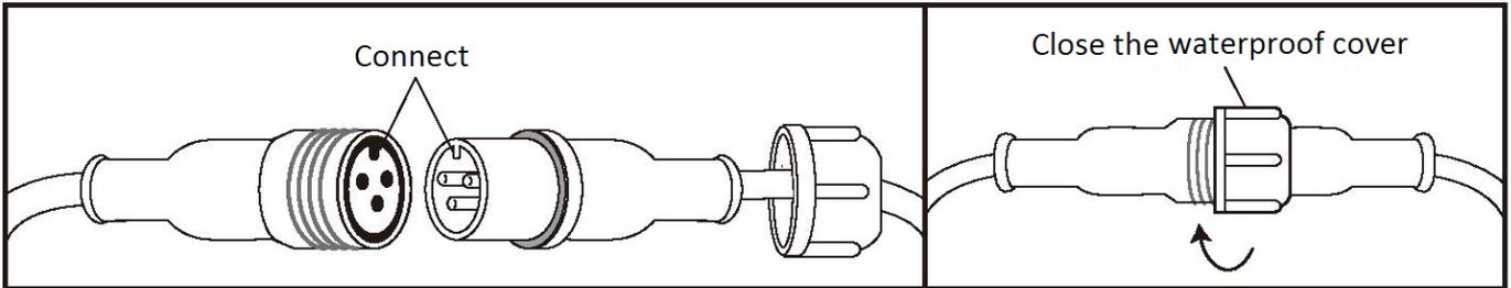
4. Connect the controller and Wave pump.
